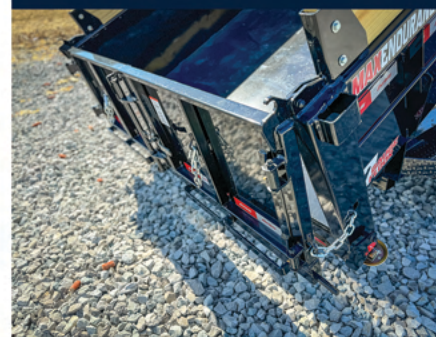
COMBO-STYLE REAR GATE (SPREADER & BARN DOORS)
