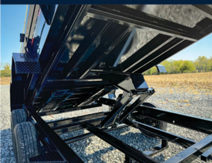
STURDY SCISSOR HOIST W/ 45° DUMP ANGLE
